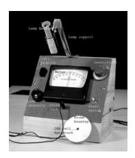
The heart of the photometer is a cadmium sulfide (CdS) cell. A CdS cell is a solid-state device
