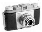
This is a 35mm "plain vanilla" camera for beginners made from 1950 through 1954. It is a pure American made camera. The lens is a Kodak coated Anaston 51mm F4.5 that collapses inside the body. The shutter is not self-cocking. Focusing is by a rotation of the lenses front element after first measuring or estimating the camera to subject distance. The body is all-
