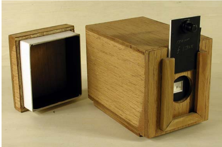
The author’s wooden pinhole camera with f/328 150mm pinhole, sliding shutter and removable back. Not shown is the tripod socket.
