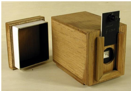
The author's f/328 150 mm pinhole camera with sliding shutter and removable back.
