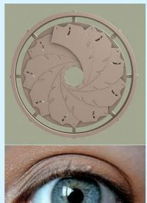
Therefore, f/16 is said to be 8 times 'slower' than f/4 because it is 8 times larger than f/16 in terms of lens opening surface and requires 8 times more exposure time.. To use this information another way, an exposure of 1/30 sec @ f/4 is equivalent to 1/8 sec. @ f/8. A user friendly way to put it more is that the difference in the two exposures is 0 EV. If we maintained the 1/30 sec. exposure but changed the aperture from f/4 to f/8 the difference would be 2 EV.
